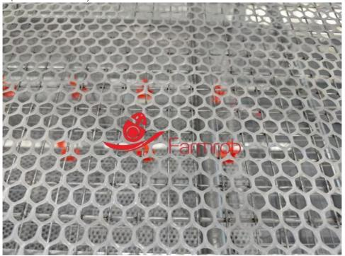
Equipped with an automatic manure removal system to keep themanure away from manures in the cage, which improves the hygienic conditions and reduce the disease rate. The belt will always keep on track. The manure from each tier of cages is carried by manure belts to the end of the house. It is then transported out of the house.
