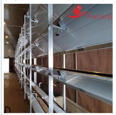
$3. The \ air \ guide \ plates \ are \ made \ of \ 30/50 mm \ insulated \ panels \ with \ an \ aluminum \ alloy \ frame.$
